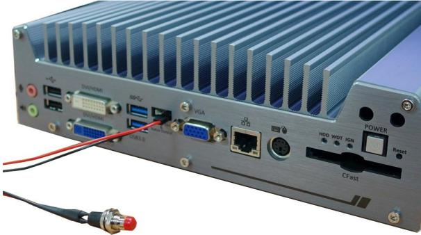
3. Push the non-latched switch will turn on the system (the PWR LED indicator on the front panel is on at the same time). Push the non-latched switch when system is on will turn off the system. If your operating system supports ATX power mode (i.e. Microsoft Windows or Linux), push the power button causes a pre-defined system behavior, such as shutdown or hibernation.
