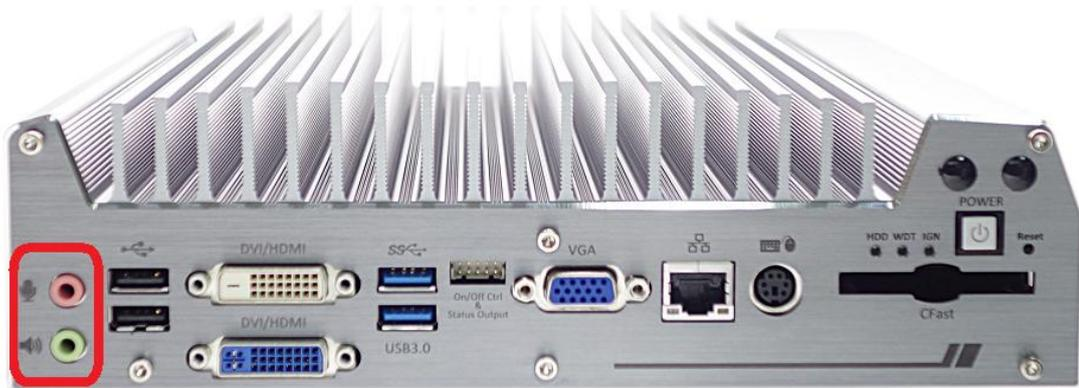
Nuvo-3616VR series provides audio function using Intel® High Definition Audio (built-in in QM77 PCH) and Realtek ALC262 Codec. There are two audio jacks on the front panel. The pink one is used for microphone input, and the green one is used for speaker output. To utilize the audio function in Windows, you need to install corresponding drivers for both Intel® QM77 PCH chipset and Realtek ALC262 Codec. Please refer to section 4.5 for information about driver installation.
