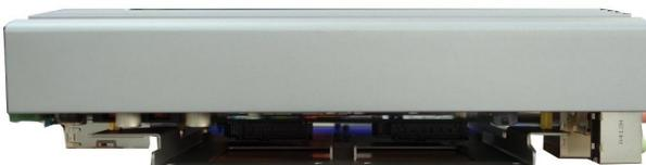
3. Gently slide the HDD/SSD drive into the Nuvo-3616VR internal HDD bracket till it's firmly connected to SATA connector.
