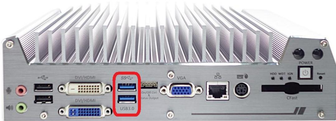
Nuvo-3616VR series offers two USB 3.0 (SuperSpeed USB) ports on its front Interface. By BIOS default, these USB ports are operated in xHCI (eXtensible Host Controller Interface) mode and are compatible with USB 3.0, USB 2.0, USB 1.1 and USB 1.0 devices. Legacy USB support is also provided so you can use USB keyboard/mouse in DOS environment. To use USB 3.0 ports in Windows 7, you need to install USB 3.0 driver. Please refer to section 4.5 for information of driver installation.
