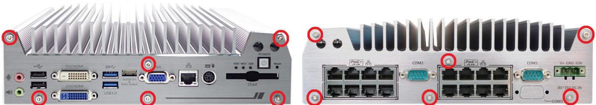
3. Remove the front panel, back panel and bottom cover to expose the PCBA with HDD bracket of Nuvo-3616VR.
