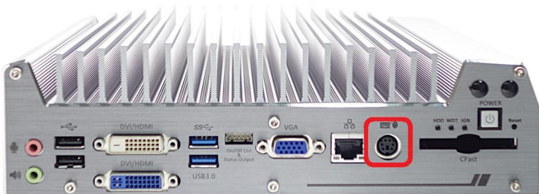
Support for legacy PS/2 keyboard and mouse on Nuvo-3616VR series is implemented using industrial-grade ITE8783 Super IO chip (-40 to 85°C). There is one 6-pin Mini-DIN connector on the front panel to provide PS/2 KB/MS signals. You shall need to use a Y-cable to connect PS/2 keyboard and mouse at the same time.
