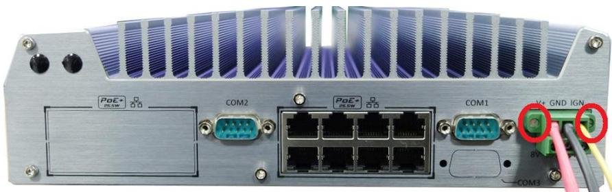
\* Neusys provides the option of 280W AC/DC (24V/11.67A) adapter for powering both Nuvo-3616VR/3608VR system and external PoE devices.
