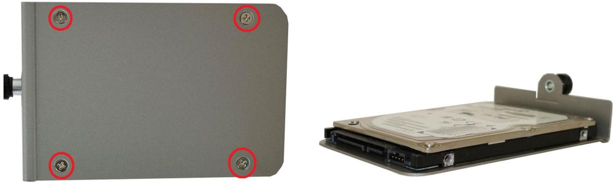
3. Gently slide the HDD tray assembly into the slot on the side of Nuvo-3616VR till it's firmly connected to SATA connector.
