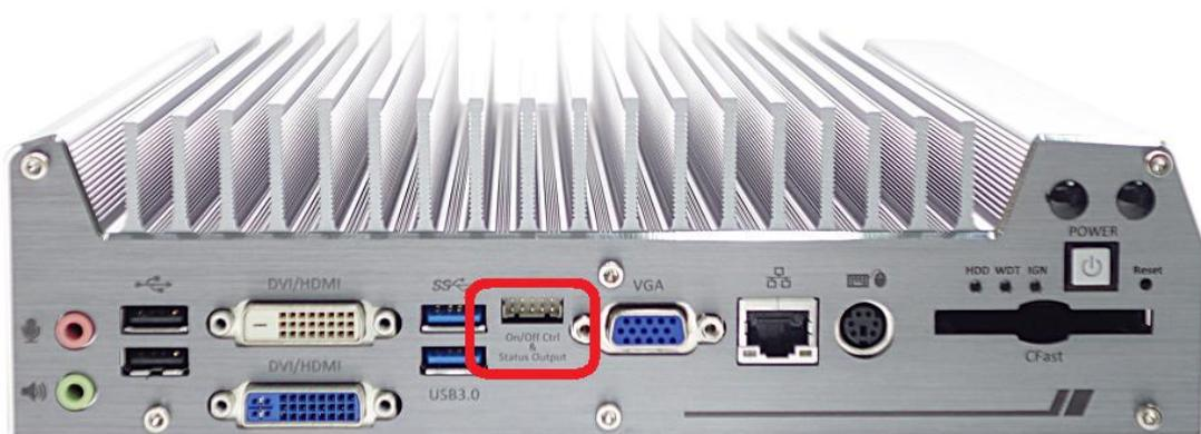
For an application which places Nuvo-3616VR series inside a cabinet, it's useful to control the on/off of the system via an external switch, as well as check how the system's running via some external LED indicators. Nuvo-3616VR series provides a 2x5, 2.0mm pitch wafer connector on the front panel for this purpose.
