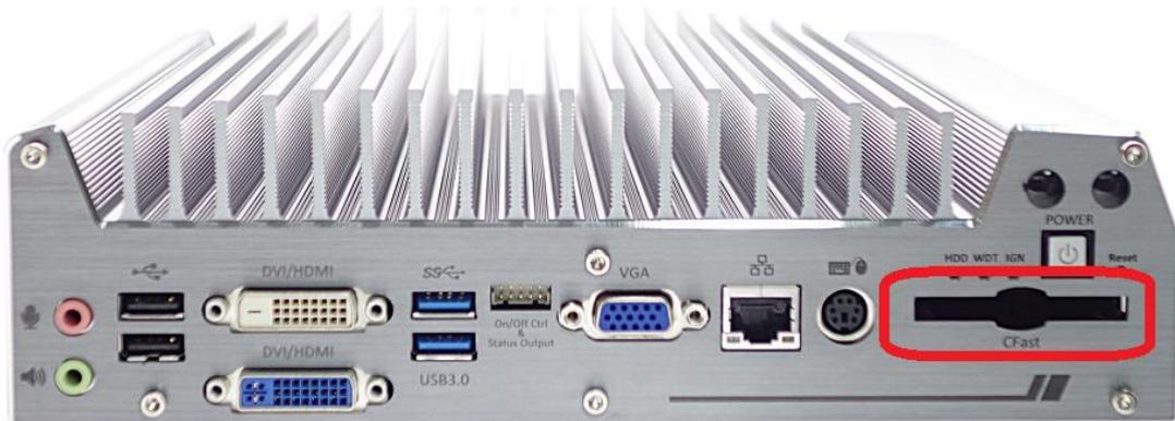
Nuvo-3616VR series provides a CFast socket on the front panel. CFast is a new interface for portable storage device. It shares a similar form-factor as CompactFlash but leverages Serial ATA interface to offer higher data transfer rate. The CFast socket on Nuvo-3616VR series is a push-push type. You can insert and push a CFast card to the end to install it, and push the installed CFast card again to eject it.
