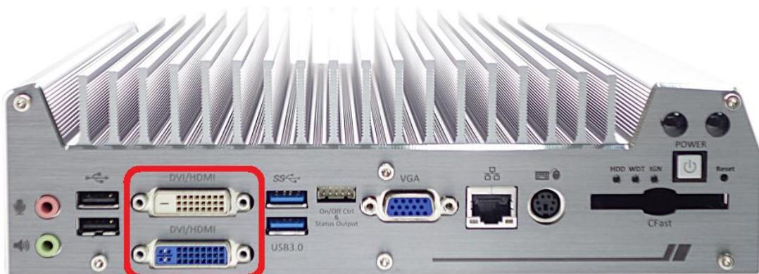
Nuvo-3616VR series has multiple display outputs on its front panel for connecting different displays according to your system configuration. DVI/HDMI transmits graphics data in
