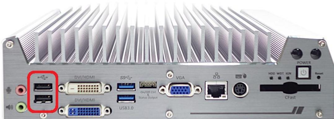
In addition to two USB 3.0 ports, Nuvo-3616VR series provides another two USB 2.0 ports on the front panel. By BIOS default, these USB 2.0 ports are operated in EHCI (Enhanced Host Control Interface) mode and are compatible with USB 2.0, USB 1.1 and USB 1.0 devices. Legacy USB support is provided so you can use USB keyboard/mouse in DOS environment.
